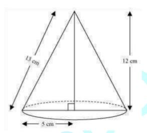
When right-angled  $\triangle$ ABC is revolved about its side 12 cm, a cone with height (h) as 12 cm, radius (r) as 5 cm, and slant height (l) 13 cm will be formed.
