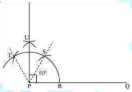
We have,  $\angle$  SPQ =  $\angle$  TPS = 60°. In (iii) and (iv) steps of this construction, PU was drawn as the bisector of  $\angle$  TPS.
